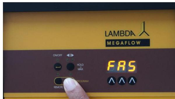
**Figure 1-8** The display will show the default mode **FAS** or the last used mode (**FAS / SLO**).
