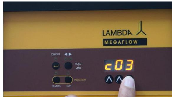
**Figure 2-18** If you wish to repeat the same program 3 times, increase the cycle number to “c03” by pressing the buttons  $\wedge \wedge \wedge$  below the display (from 0 to 99 cycles). The program can be repeated up to 99 times, indicated by “c99”. If 0 is entered for the cycle number “c00”, the program will run continuously (infinite loop).
