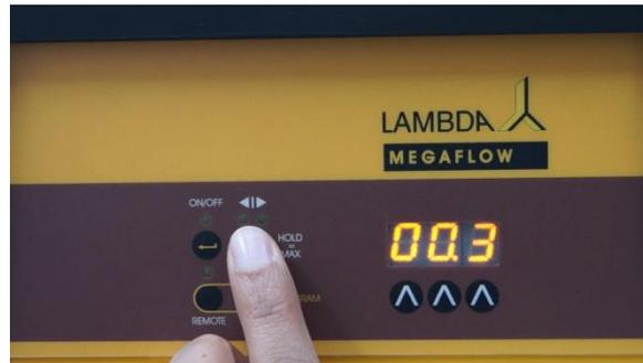
**Figure 2-14** Press ◀▶ button, to set the time resolution.
